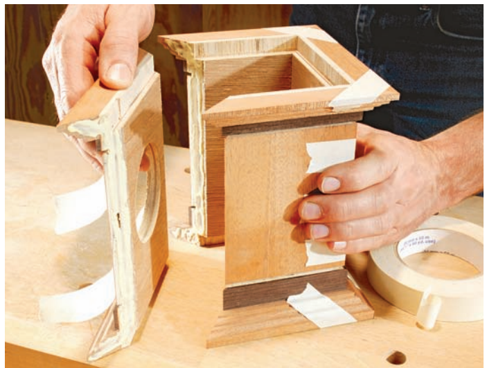
10 Assemble the sides with glue and masking tape. Pull the masking tape tight and check that the miters align tightly.
